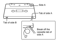
If you later want to reuse the tape for recording, cover the broken tab with adhesive tape.
