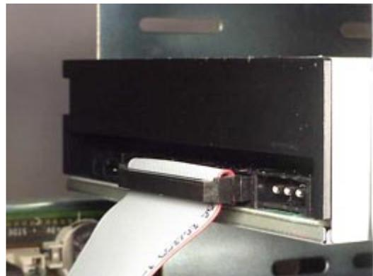
**Power Cable** - Connect an internal computer power supply cable to the power socket at the back of the DVD-ROM drive. One side of the plug has chamfered edges, so the power connector fits only one way. Push plug completely into the socket making sure the plug fits correctly.
