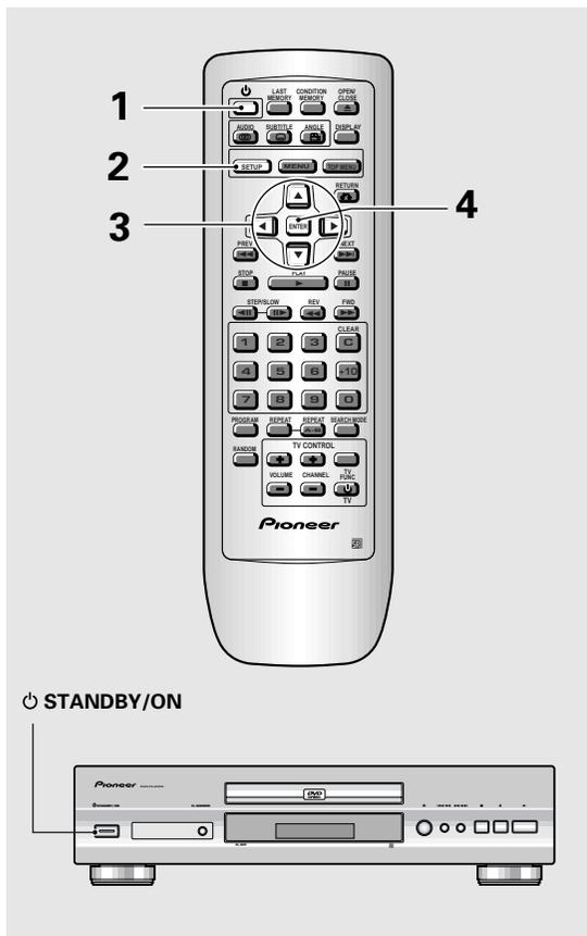
**1 Press** **⏻ STANDBY/ON** on the front panel (**⏻** on the remote control).
