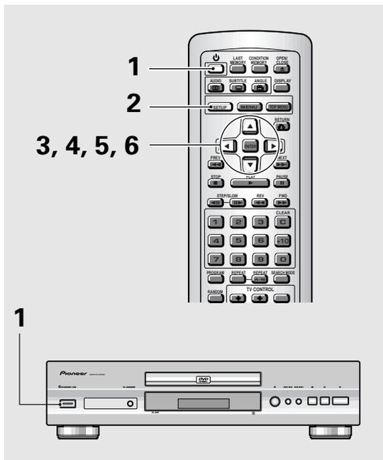
**1** Press **⏻ STANDBY/ON** on the front panel (**⏻** on the remote control)
