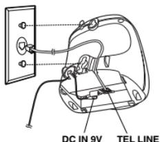
For direct wall mounting, align the base's keyhole slots with the mounting screws and slide the base downward to secure it.
