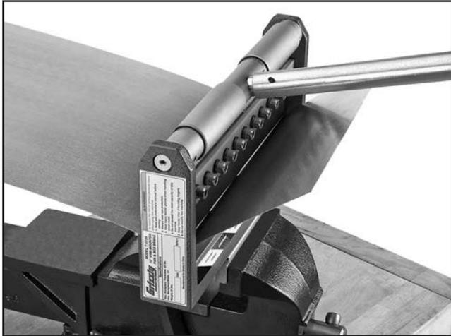
**Figure 7.** Example of a 90° bend.
