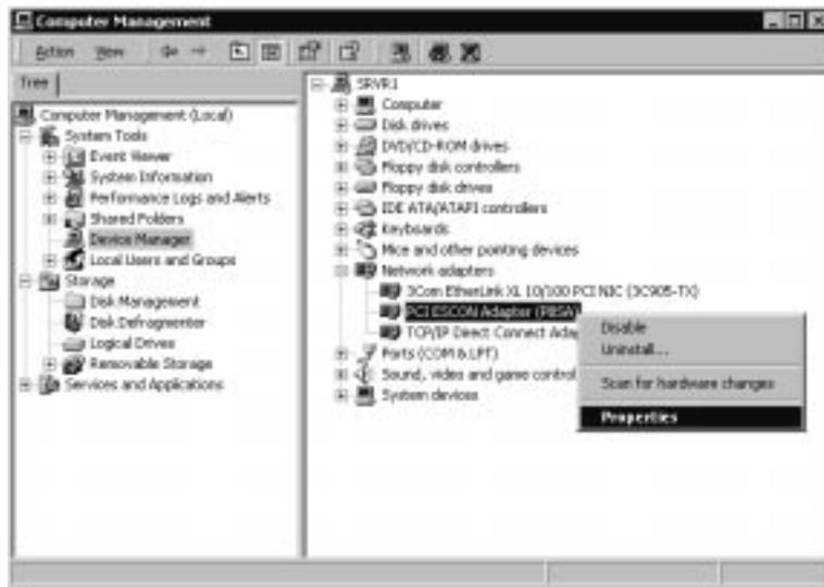
Figure 4-3. Accessing ESCON Configuration in Windows 2000
