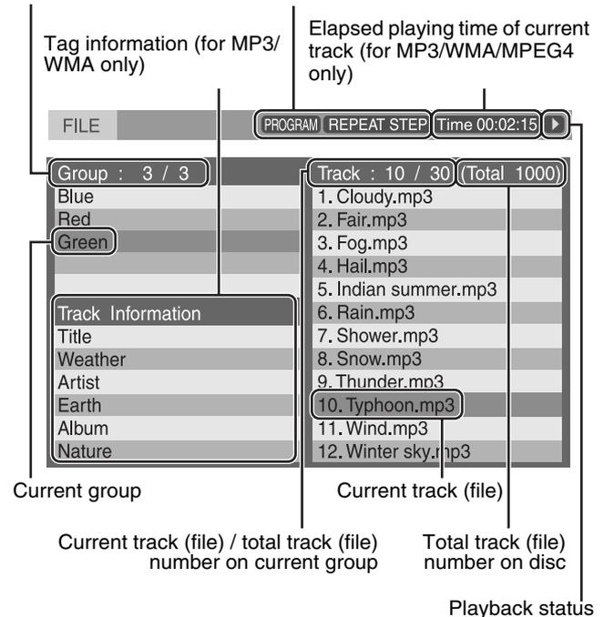
The file control display appears automatically during playback (MP3/WMA) or while stopped.
