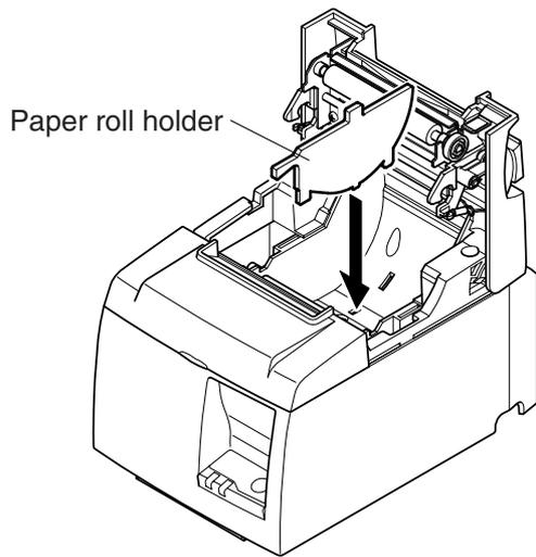
**Note:** When using a paper roll with an 57.5 mm width, install the paper roll holder in the groove in the printer.
