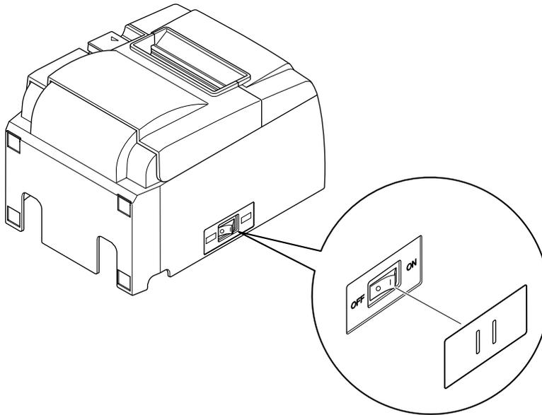
The power switch can be turned ON (I) and OFF (O) by inserting a narrow instrument (ball pen etc.) in the holes in the switch cover.
