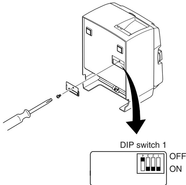
When the printer is shipped, DIP switch 1-4 is set to OFF; all of the other switches are set to ON.
