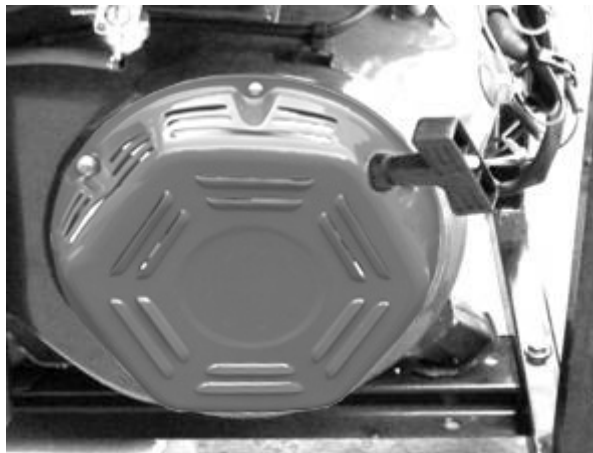
Figure 6 - Pull-cord for starting the engine.
