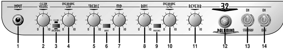
**1. Input:** Connect your instrument here by means of a shielded signal cable.
