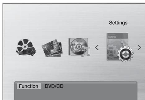
1. Press the **POWER** button in NO DISC mode, or During playback, press the **STOP** button twice.
