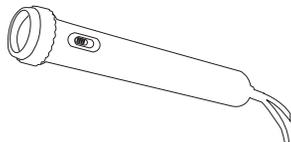
Micro Forever Flashlight will provide you with five to seven minutes of light when charged for 30 seconds. If the unit is completely drained of energy, you should give the unit 90 shakes—or about 30 seconds of shaking at 3 shakes per second—to fully charge its capacitor.
