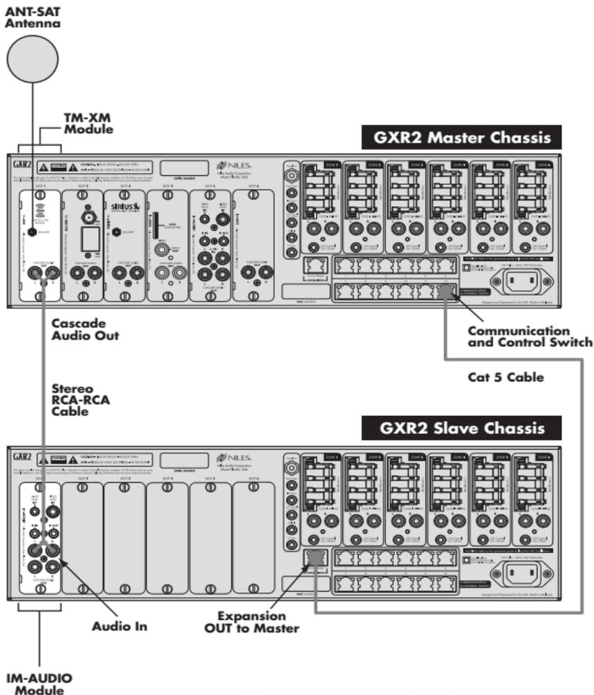
Figure 7. Expanded System with Cascade Audio
