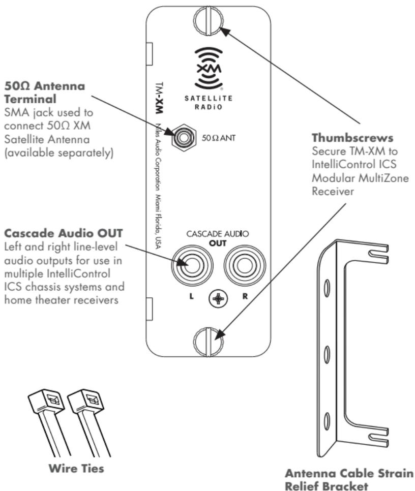
**Figure 1.** IntelliControl ICS TM-XM Module
