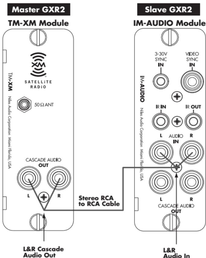
Figure 6. Cascade Audio Connections
