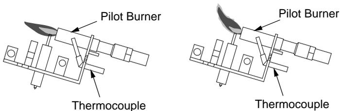
**Figure 31 - Correct Pilot Flame Pattern (Propane/LP Shown)**
