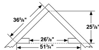
Figure 7 - Rough Opening for Installing in Corner
