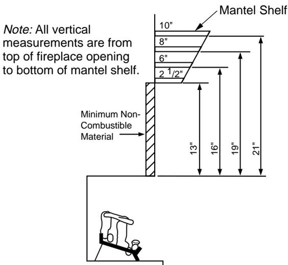
Figure 9 - Minimum Mantel Clearances for Built-In Installation
