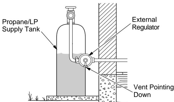
**Figure 20 - External Regulator with Vent Pointing Down**
