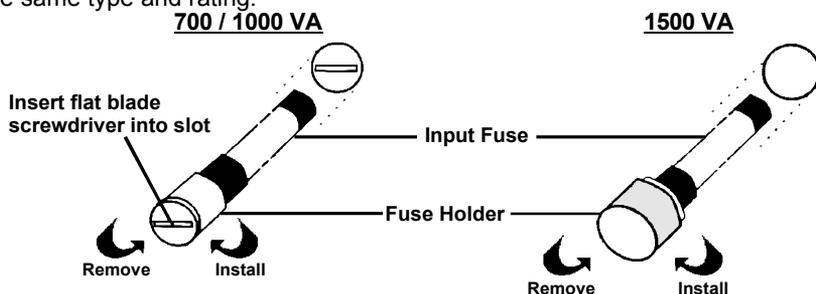
1. Remove the fuse holder by inserting a flat blade screwdriver into the slot (twist by hand for the 1500 VA model) and rotating counter-clockwise to remove.
