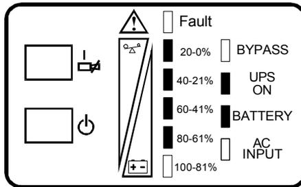
Figure 2 – Battery Mode Operation at 61-80% battery capacity
