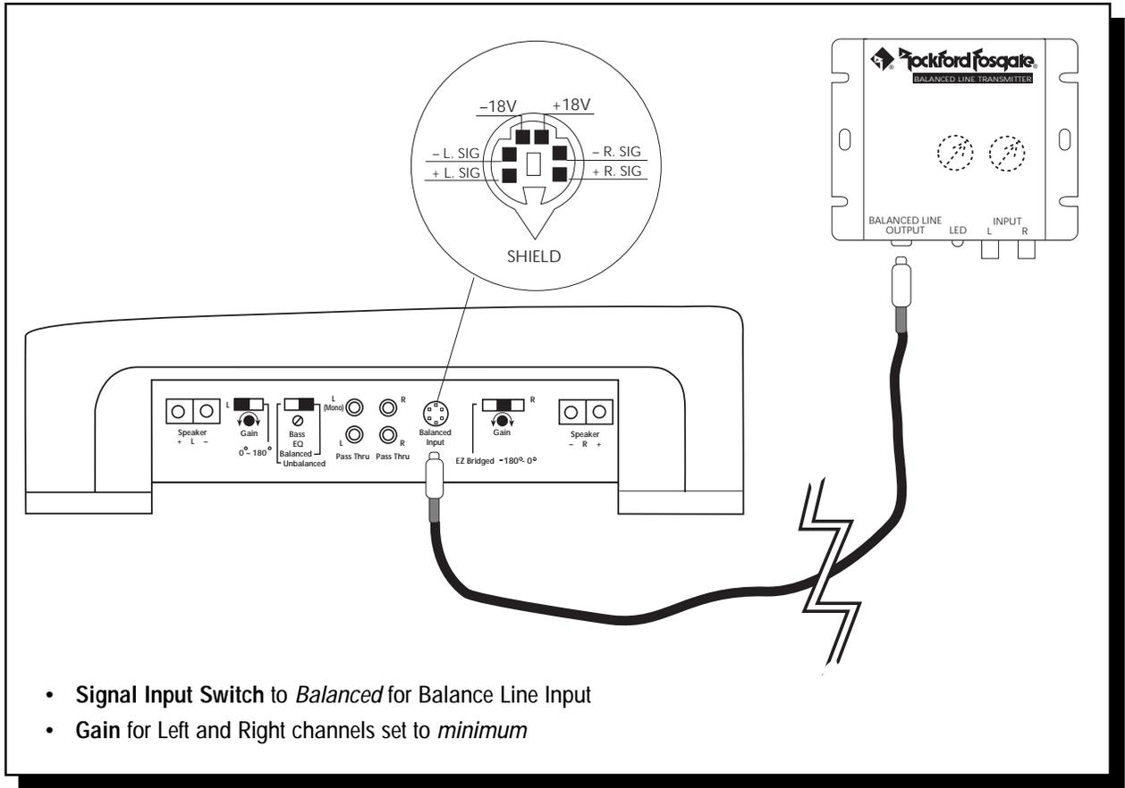
**CAUTION!!** You must turn the gain controls to minimum when using the Balanced Line Transmitter. If the input gains need to be adjusted, this can now be done in the Balanced Line Transmitter.
