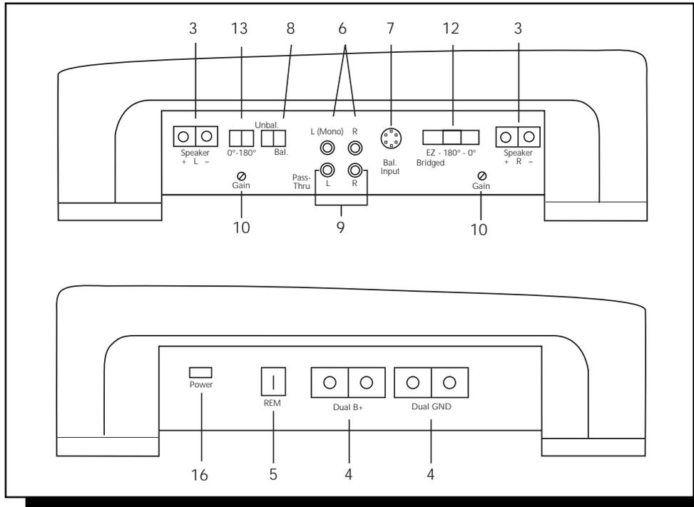
3. **Speaker Terminals** – The heavy duty, gold-plated terminal block connectors (+ and –) will accept wire sizes from 8 AWG to 18 AWG. These gold-plated connectors are immune to corrosion that can cause signal deterioration.
