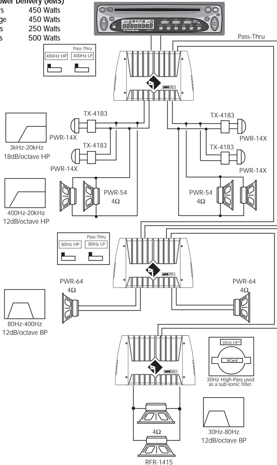
• A sub-sonic filter is a high-pass filter that limits the input signal below a certain motion below that frequency. At very low frequencies a woofer has no output, just motion. If you try to drive this woofer at these lower frequencies, the woofer could self-destruct. Please refer to the crossover section of the manual or see your local Authorized Rockford Fosgate Dealer for more information.
