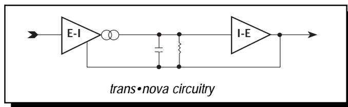
The resulting design utilizes an output stage with a simpler gain structure and a shorter total signal path than conventional high voltage (bi-polar) designs. The number of stages is reduced from five or more to three. The output stage is further refined into a trans-impedance stage (current to voltage converter) to achieve a short loop (fast) negative feedback. The output stage is driven cooperatively by a transconductance stage (voltage to current converter).
