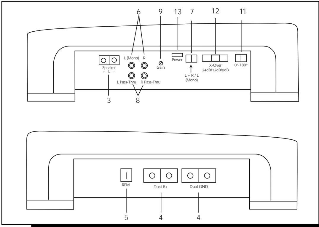
3. **Speaker Terminals** – The heavy duty, gold-plated terminal block connectors (+ and –) will accept wire sizes from 8 AWG to 18 AWG. These gold-plated connectors are immune to corrosion that can cause signal deterioration.
