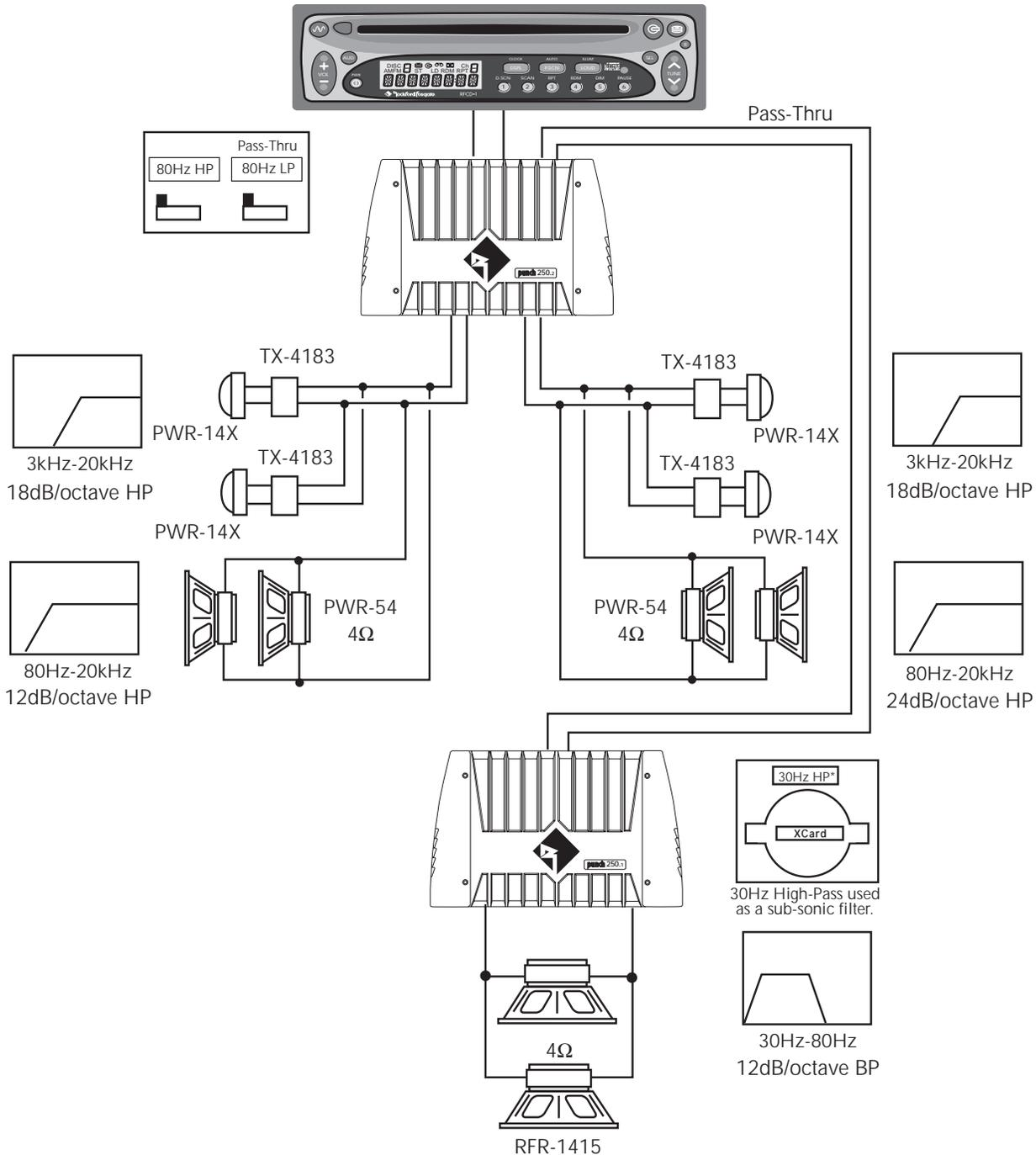
• A sub-sonic filter is a high-pass filter that limits the input signal below a certain motion below that frequency. At very low frequencies a woofer has no output, just motion. If you try to drive this woofer at these lower frequencies, the woofer could self-destruct. Please refer to the crossover section of the manual or see your local Authorized Rockford Fosgate Dealer for more information.
