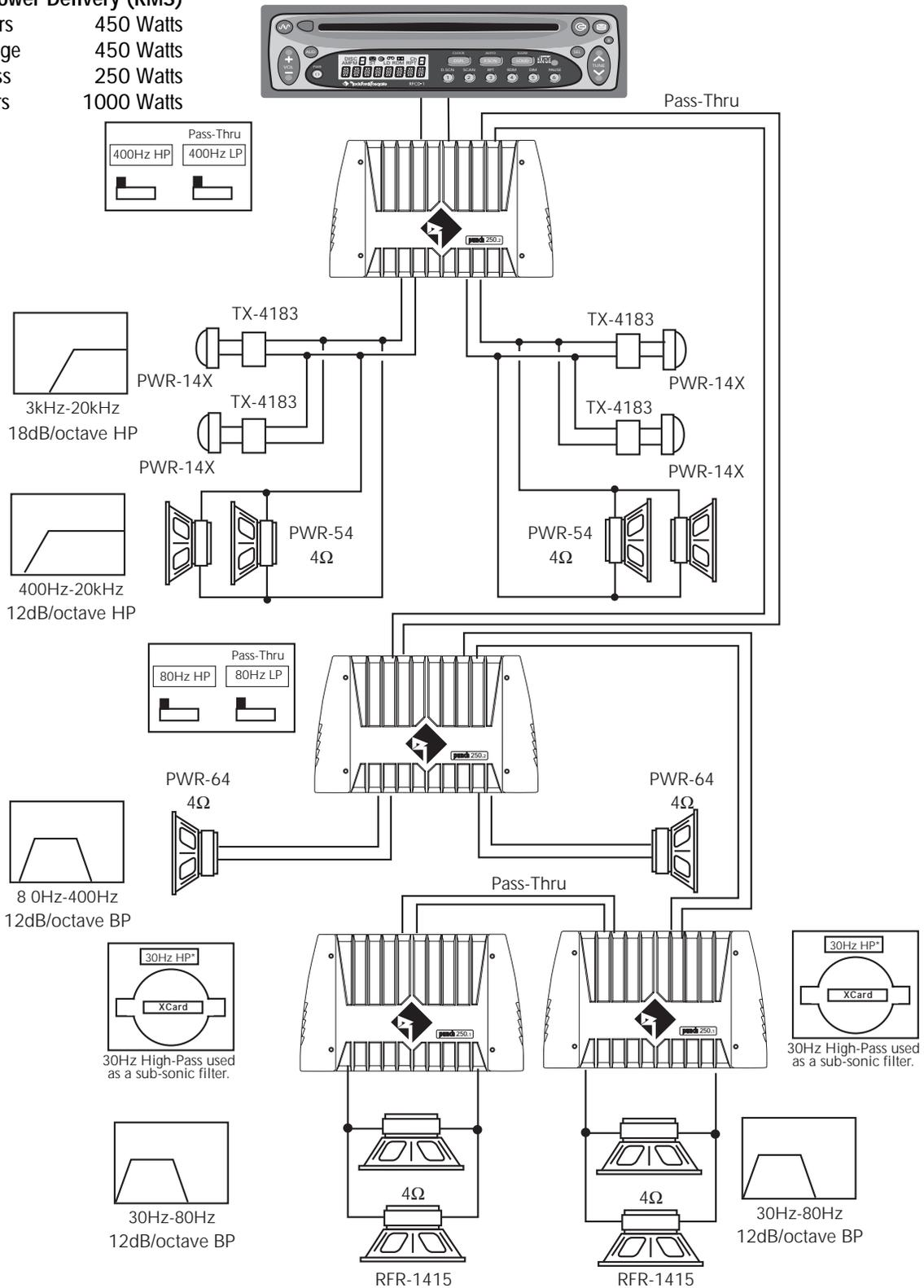
• A sub-sonic filter is a high-pass filter that limits the input signal below a certain motion below that frequency. At very low frequencies a woofer has no output, just motion. If you try to drive this woofer at these lower frequencies, the woofer could self-destruct. Please refer to the crossover section of the manual or see your local Authorized Rockford Fosgate Dealer for more information.
