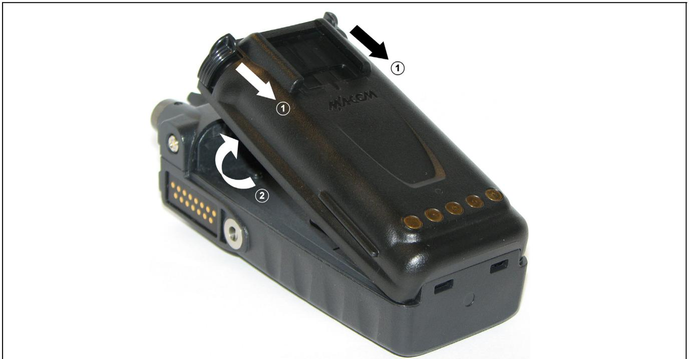
Figure 4-1: Removing the Battery Pack
