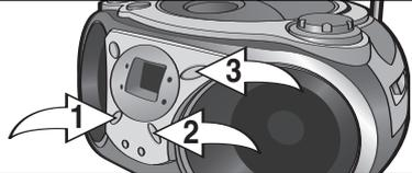
To start from a specific track, while in the stop mode, locate the track using the Skip/Search ◀◀ 1 or ▶▶ 2 button, then, within five seconds, press the PLAY/PAUSE (▶/||) button 3 to start playback from the track selected. The PLAY/PROG indicator will light.
