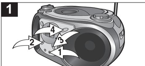
**To repeat a single track**, press the REPEAT button ① once while in the Stop mode; the Repeat indicator will blink. Press the Skip/Search ◀② or ▶③ button to select the specific track that you wish to repeat. When the desired track number appears in the display, within five seconds, press the PLAY/PAUSE (▶/||) button ④ to begin playback. The PLAY/PROG indicator will light and the specific track you selected will be repeated continuously.
