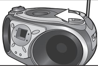
Open the CD Compartment door by pressing the OPEN/CLOSE area. Place a CD on the center spindle, with the printed label side facing up. Close the CD Compartment door; the total tracks will appear in the display.
