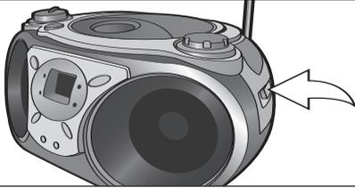
Slide the Function switch to the CD position to turn the unit on and select CD mode; the POWER ON indicator will light.
