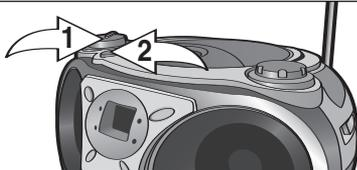
Adjust the VOLUME control 1 and BASS BOOST button 2 as desired. Press the BASS BOOST button 2 to the "in" position to enhance the bass sound; the BASS BOOST indicator will light.
