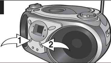
Repeat steps 3 and 4 to program the other desired tracks in sequence. When the program memory is full, the unit will run through the programmed tracks in the display and then revert to "01".
