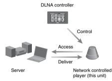
The unit can play audio content stored on the server in MP3, Linear PCM, WMA and AAC\* formats. Audio content with DRM (Digital Rights Management) copyright protection cannot be played on this unit.
