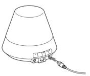
**3** Plug the AC power cord to a wall outlet (the mains).
