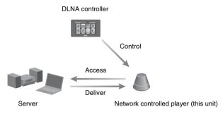
You can enjoy audio content using only this unit and a computer by using the computer as both server and controller. Windows 7 has to be installed on your computer to use this function. For details, refer to page 20.
