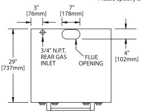
Commercial cooking equipment requires an adequate ventilation system. For additional information, refer to the National Fire Protection Association's standard NFPA96...
