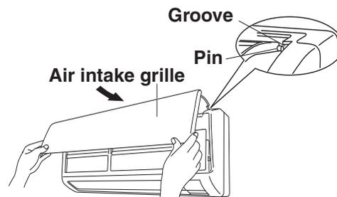
3. To attach the air intake grille to the indoor unit, press its bottom right and left corners as well as its bottom center into place.
