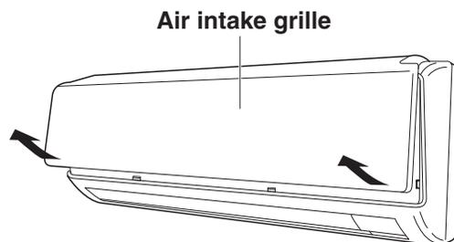
2. Remove the filter attached to the rear of the air intake grille.
