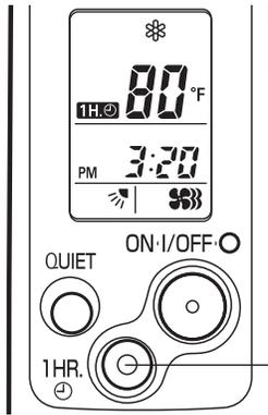
This function causes the unit to operate for one hour and then stop, regardless of whether the unit is on or off when this button is pressed. The **1H.** icon in the display indicates that this function is operating.
