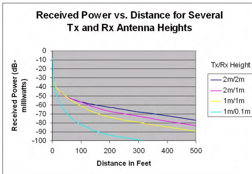
FIG. 8 Antenna Height Influence on Received Signal Strength
