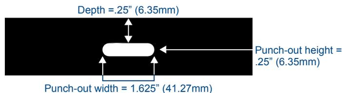
**FIG. 7** ANT-BDG - Slot Punch dimensions
