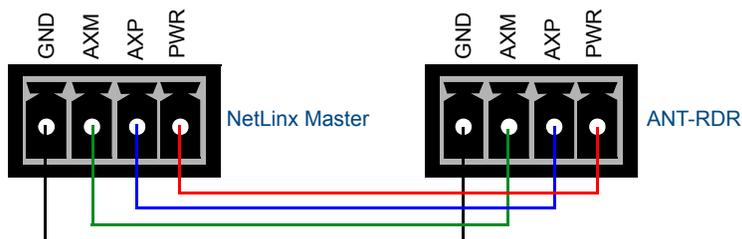
FIG. 11 AXlink data/power connections
