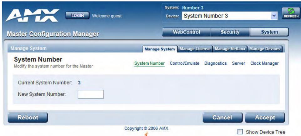
FIG. 15 Manage System page - Manage System tab
