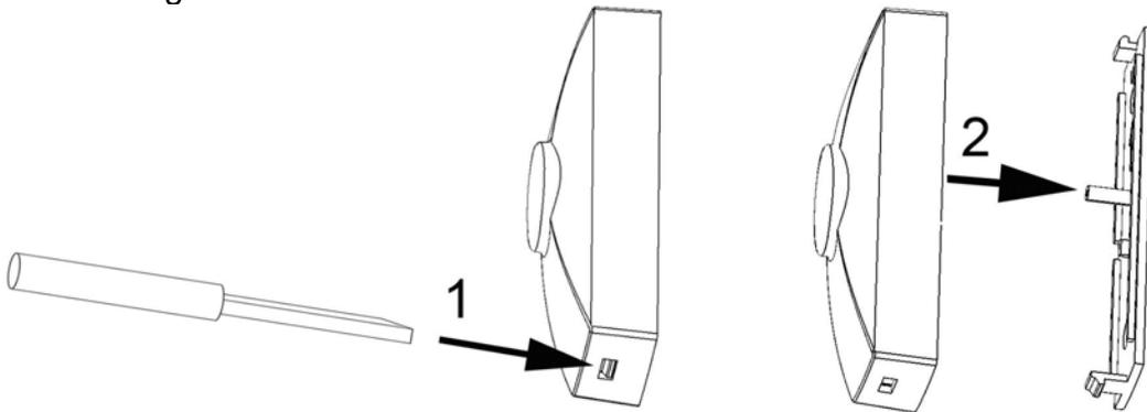
b. Replacing the back cover
