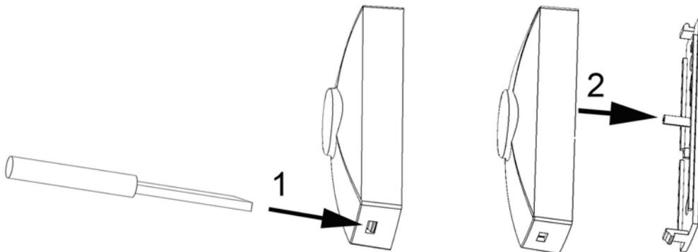
3. Locate the House Security Code door and screw located on the back of the AC Chime. Remove the screw and take off the door.
