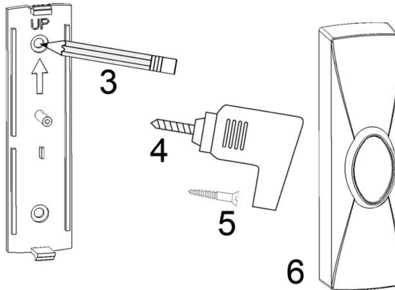
4. Drill two holes with 3/32" drill in marked locations.
