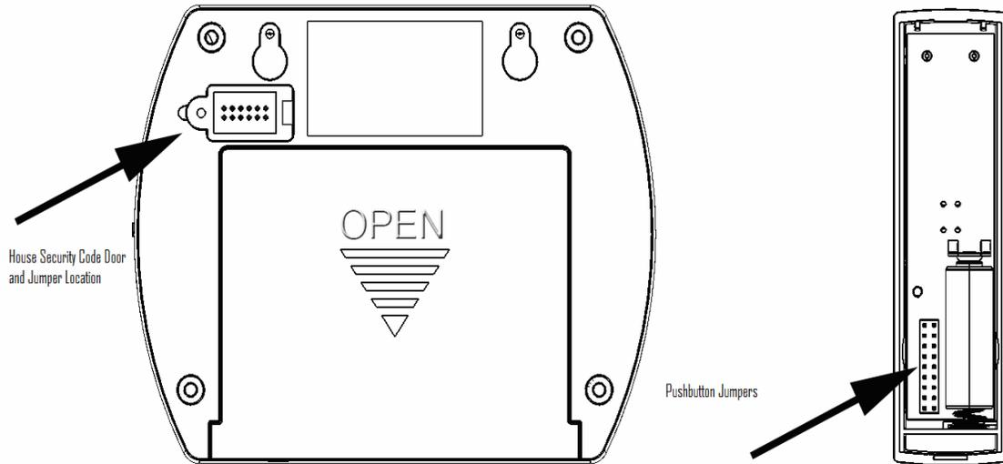
The chime and pushbutton must be set to the same house security code for the combination to operate together.
