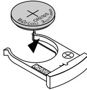
**3** Insert the battery holder into the remote control and push in until the battery holder closes with a "click" sound.
