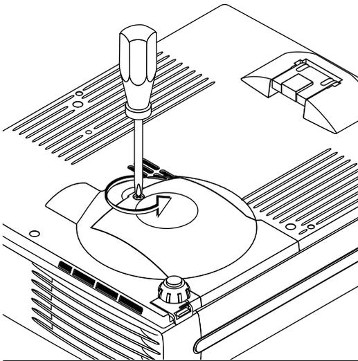
(2) Open the lamp cover a little, then pull it in the direction of the arrow and remove it.
