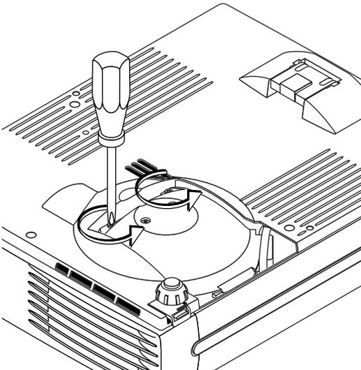
(2) Grasp the lamp cartridge's handle and pull upward to remove the lamp cartridge.
