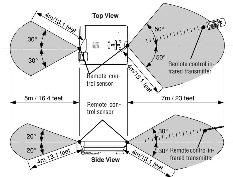
\* The position of the remote control sensor at the front of the main unit will differ depending on the projector model.
