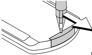
**2** Remove the old battery and install a new button battery with (+) side facing upward in the battery holder.
