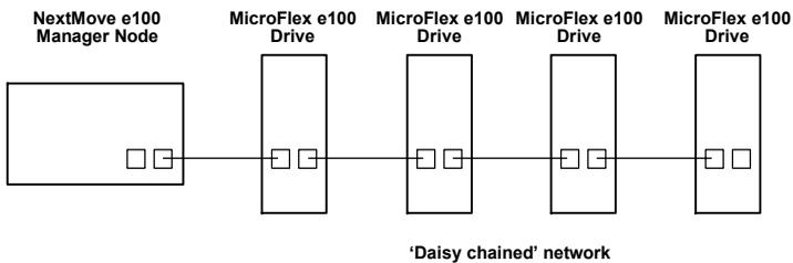
Figure 36 - Simple daisy-chained EPL network
