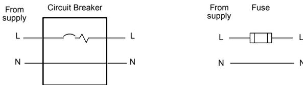
Figure 4 - Circuit breaker and fuse, single-phase
