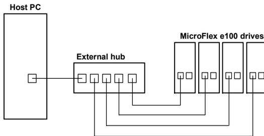
Figure 34 - Connecting to drives using TCP/IP in standard Ethernet mode
