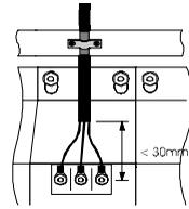
Figure 53 - Earthing/grounding cable shields
