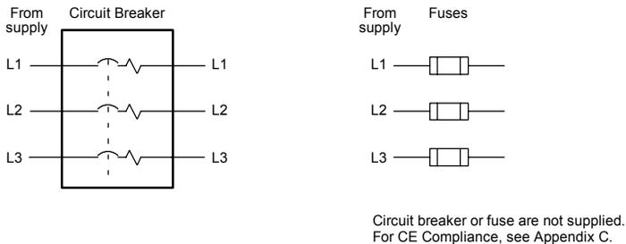
Figure 5 - Circuit breaker and fuse, three-phase
