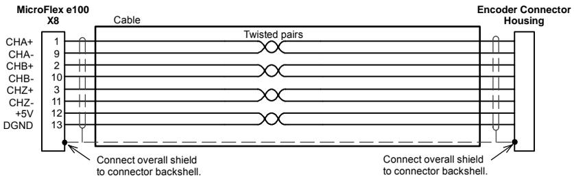
Figure 54 - Encoder signal cable grounding
