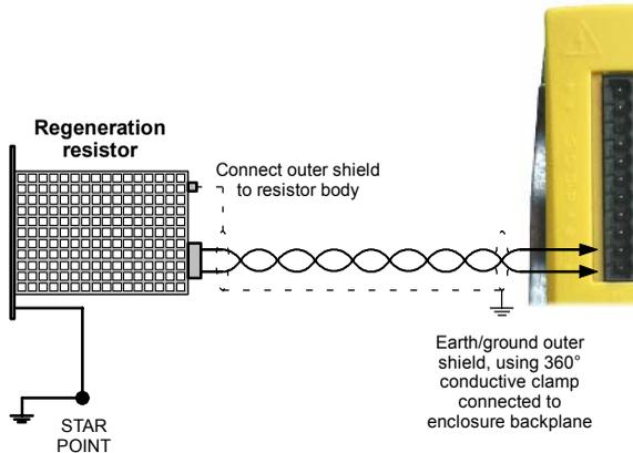
Figure 11 - Regeneration resistor connections
