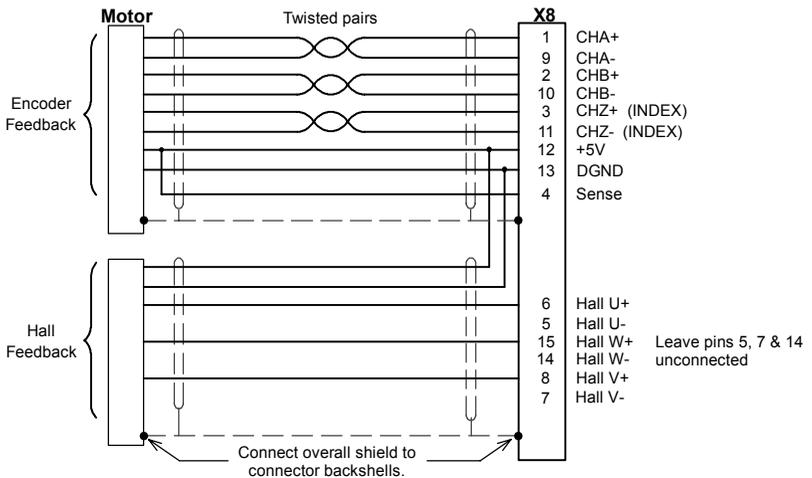
Figure 17 - Encoder cable connections - linear motors
