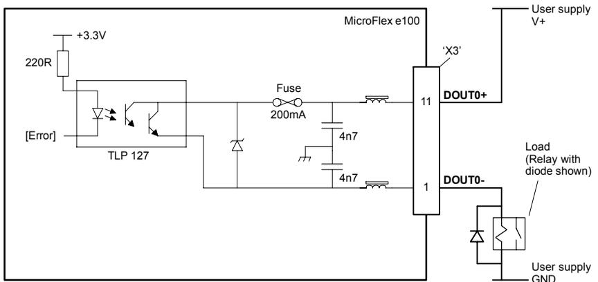
Figure 30 - DOUT0 output circuit
