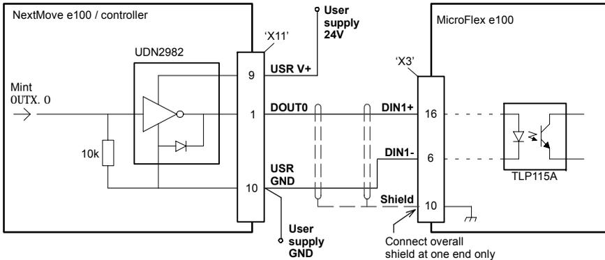
Figure 29 - Digital input - typical connection from a Baldor NextMove e100
