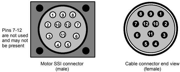
**Figure 19 - Baldor motor SSI feedback cable pin configuration**
