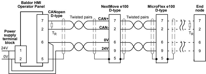
**Figure 38 - Typical CANopen network connections**
