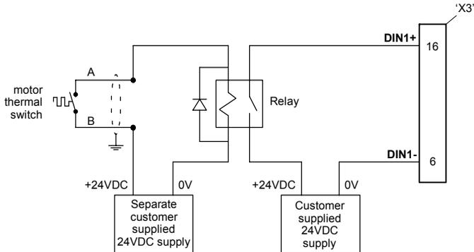
**Figure 9 - Motor thermal switch circuit**
