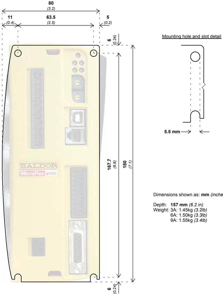
Figure 1 - Mounting and overall dimensions
