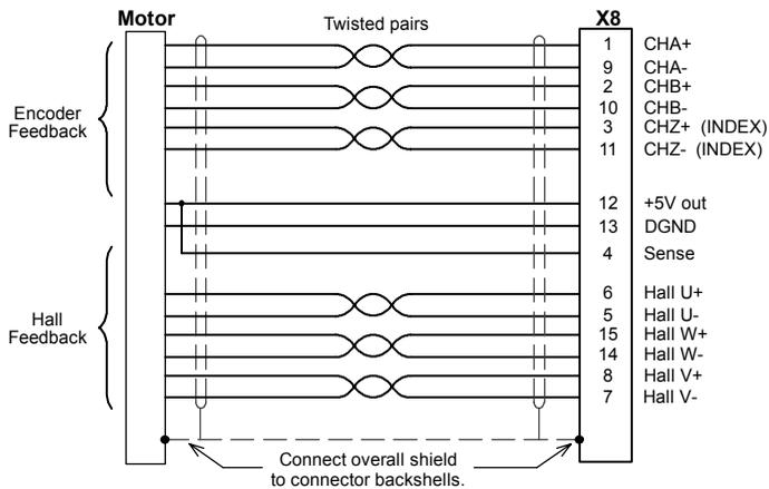
Figure 14 - Encoder cable connections - rotary motors
