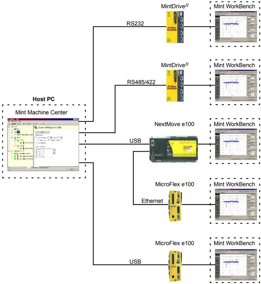
Figure 42 - Typical network visibility provided by Mint Machine Center
