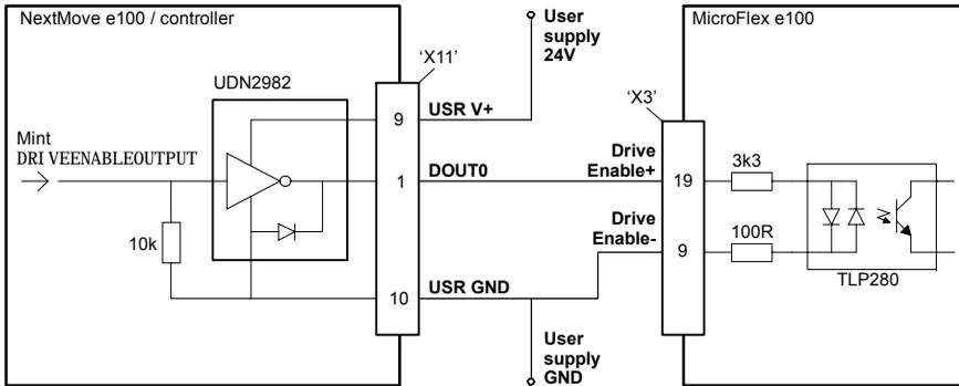
Figure 25 - Drive enable input - typical connection from a Baldor NextMove e100
