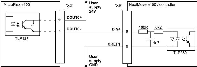
Figure 31 - DOUT0 - typical connections to a Baldor NextMove e100
