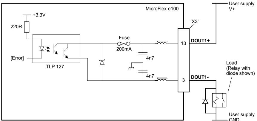
Figure 32 - DOUT1 output circuit
