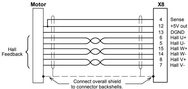
Figure 16 - Halls-only feedback cable connections - rotary motors
