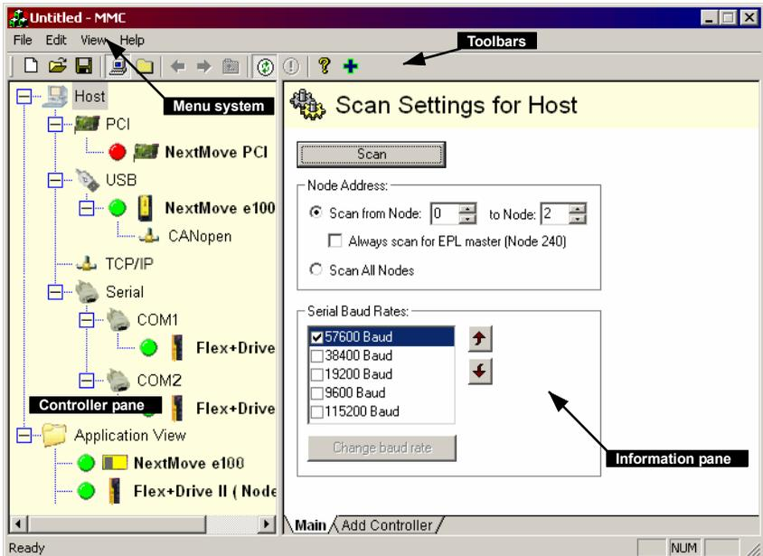
Figure 41 - The Mint Machine Center software
