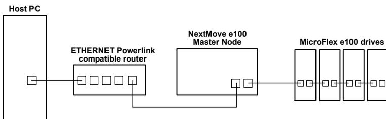
Figure 35 - Connecting to daisy-chained drives using TCP/IP and EPL mode
