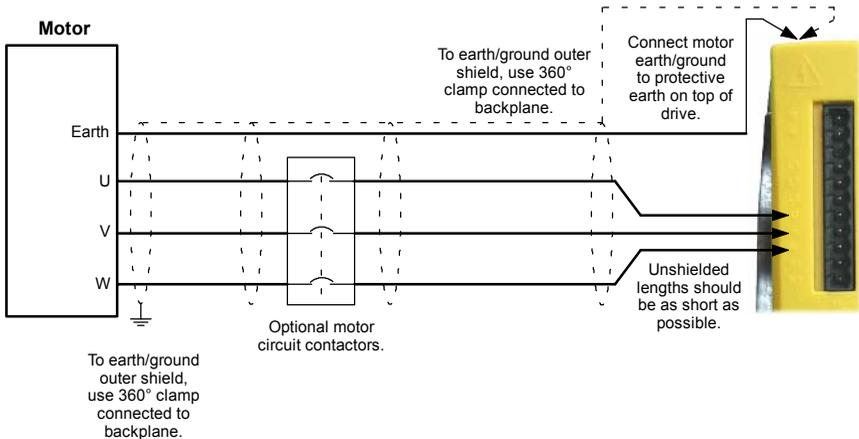
Figure 7 - Motor connections
