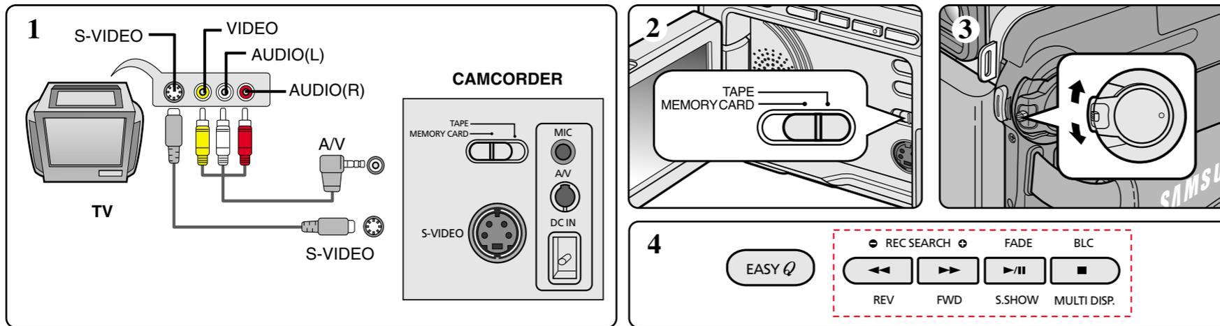
1. Connect the camcorder to a TV with the AUDIO/VIDEO cable.
