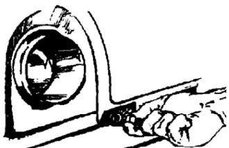
**9.** Remove the red cap from the gas pipe. Move the dryer into its final position.
