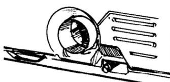
The exhaust outlet is located at the bottom center back of the dryer.
