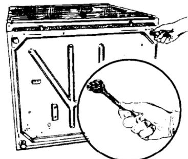
Use a 1" wrench or socket to finish turning the legs until you reach the diamond mark.
