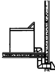
The exhaust duct can be routed up, down, left, right or straight out of the back of the dryer. Detailed space requirements can be found in "Recessed and closet installation instructions" on the back cover.
