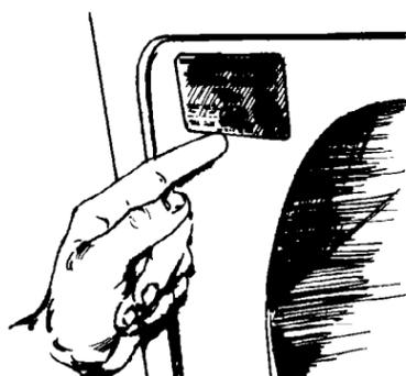
**A.** First make certain that this dryer is equipped with the correct burner for the particular type of gas in the home. Burner information will be found on the serial/rating plate in door well of the appliance. If this information does not agree with the type of gas available, see your dealer.
