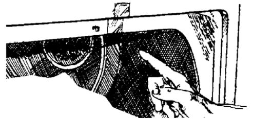
3. Remove the tape that holds the drum to the cabinet. (Some dryer drums are not taped for shipping.) Move the drum by hand to make certain all tape has been removed. Wipe the interior of the drum thoroughly with a damp cloth before using the dryer. Remove the tape from the lint screen.
