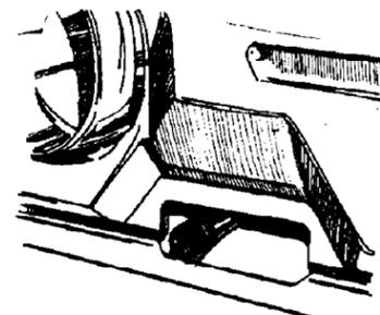
**F.** If local codes permit, it is recommended that new flexible metal tubing, design certified by the American Gas Association, be used for connecting the appliance to the gas supply line. (The gas pipe which extends through the lower rear of the appliance has 3/8-inch male pipe thread.)
