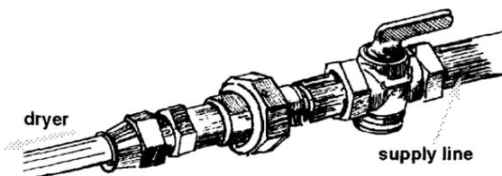
**11.** Open the shutoff valve in the gas supply line.
