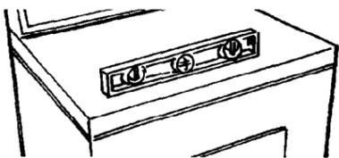
**8.** Move the dryer close to its final location. To make sure the dryer is level, take a carpenter's level and place it on the top of the dryer, first side to side; then front to back. If the dryer is not level, adjust the legs of the dryer up or down.
