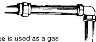
**G.** If rigid pipe is used as a gas supply line, a combination of pipe fittings must be used to obtain an in-line connection to the dryer.
