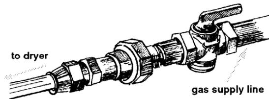
**D.** The supply line shall be equipped with a shutoff valve. This valve should be located in the same room as the dryer and should be in a location that allows ease of opening and closing. Do Not block access to shutoff valve.
