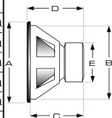
Be sure to allow 0.75 inches (19mm) for pole vent clearance on this driver.
