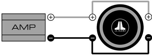
With coils wired in parallel, a dual 6Ω speaker will present a 3Ω load.
