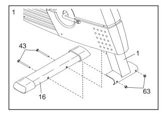
Orient the Front Stabilizer (15) as shown. Attach the Front Stabilizer to the Frame (1) with two M10 x 112mm Carriage Bolts (43) and two M10 Nylon Locknuts (63).
