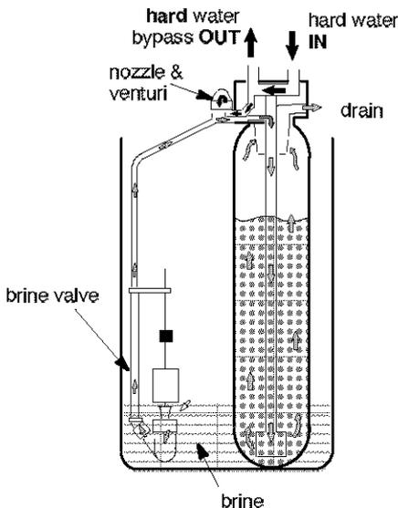
**4 BACKWASH:** During backwash, water flows UP through the resin tank (FIG. 8) at a fast rate to flush iron minerals, dirt and sediments from the bed
