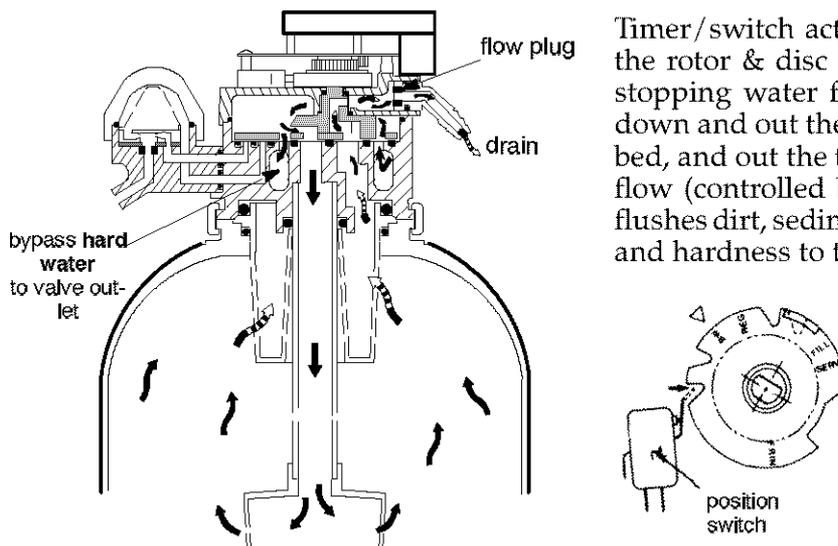
Timer/switch action again allows the motor to turn the rotor & disc to place the valve in BACKWASH, stopping water flow to the nozzle. Water is routed down and out the bottom distributor, up through the bed, and out the top distributor to the drain. The fast flow (controlled by a flow plug in the drain fitting) flushes dirt, sediments, iron deposits, remaining brine and hardness to the drain.
