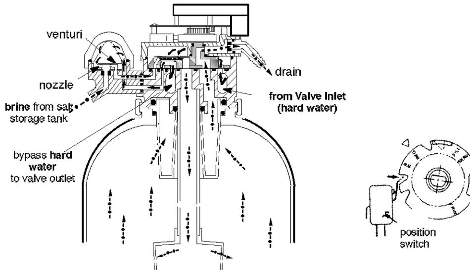
After fill, timer/switch action allows the motor to turn the rotor and disc into BRINING position. Water flow is directed to the nozzle. Suction, created by the nozzle and venturi, draws brine from the salt storage tank and injects it into the resin bed via the bottom distributor. Flow continues out the top distributor and to the drain. Hard water is available at the valve outlet.
