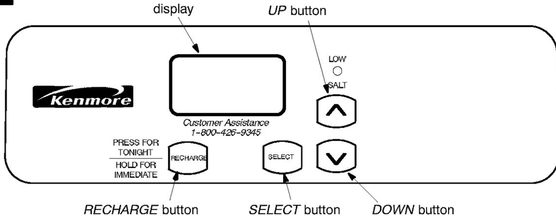
When the transformer is plugged in, a model code, and a test number (example: J1.0) show in the face plate display for 4 seconds. Then, the words *SET TIME* show in the display along with a flashing 12:00 PM.
