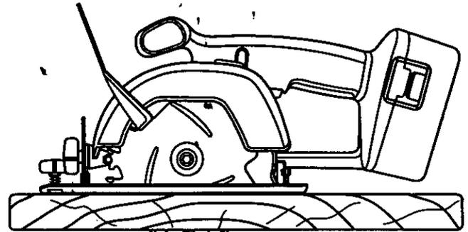
BLADE EXPOSED ON UNDERSIDE OF WORKPIECE
