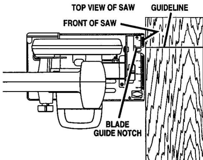
ALIGN OUTER BLADE GUIDE NOTCH ON SAW BASE WITH LINE OF CUT AS SHOWN WHEN MAKING CROSS CUTS OR RIP CUTS
