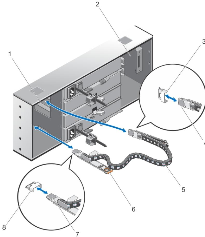
**Figure 21. Removing and Installing the SAS Chain Cable(s)**
