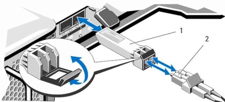
**Figure 28. Removing an SFP+ Module**
