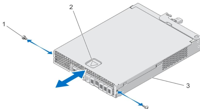
Figure 23. Opening and Closing the RAID Controller Module
