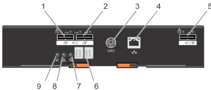
**Figure 11. MD3060e Expansion Module Features and Indicators**
