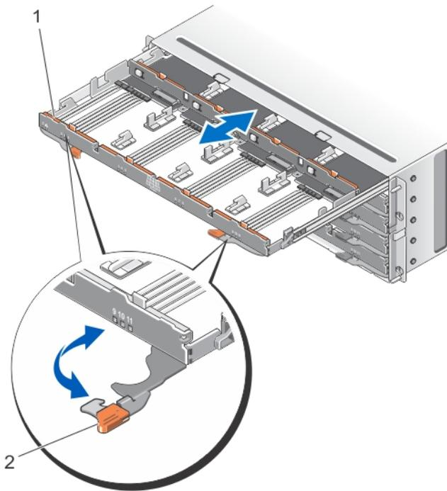
Figure 14. Opening and Closing the Physical-Disk Drawer
