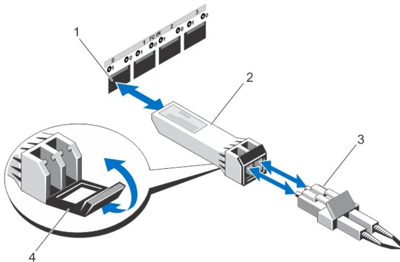
**Figure 9. Fibre Optic Cable Connection**
