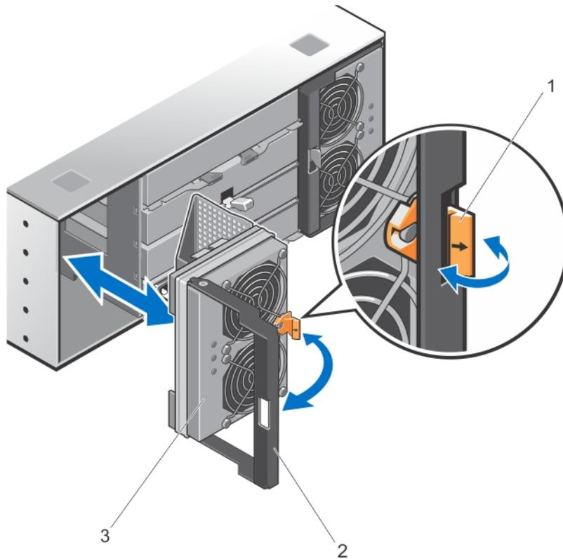
**Figure 27. Removing and Installing the Cooling Fan Module**
