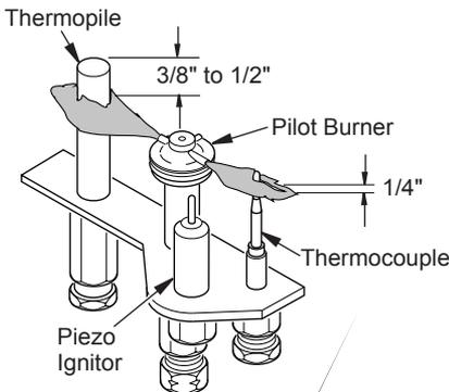
**Figure 38 - Pilot Assembly (Millivolt Ignition System)**
