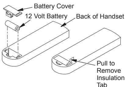
**Figure 19 - Installing Battery into Back of Handset**
