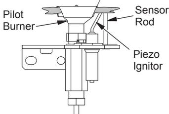
**Figure 39 - Pilot Assembly (Electronic Ignition System)**
