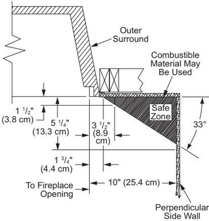
Figure 8 - Side Clearances for Combustible Mantels
