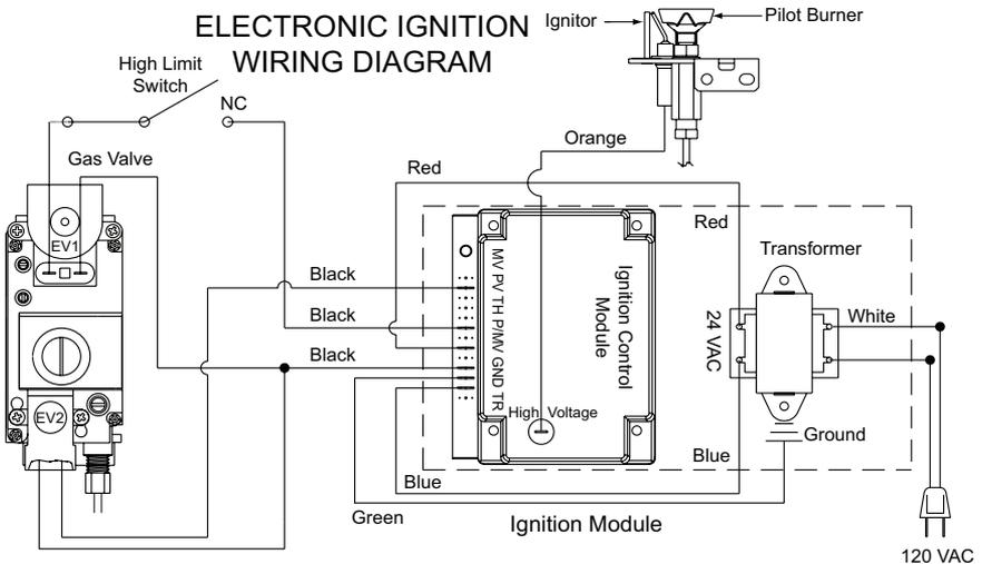
**Figure 21 - Electronic Ignition Wiring Diagram**
