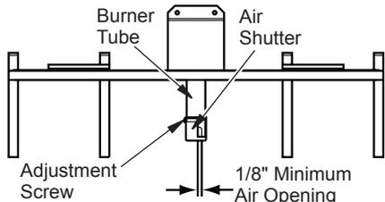
**Figure 41 - Adjusting Air Setting**
