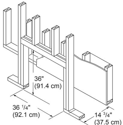
Figure 5 - Framing Clearances for Flush Wall Installation
