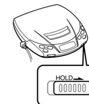
Slide HOLD in the direction of the arrow. When you press any button, "Hold" appears in the display and you cannot operate the player.
