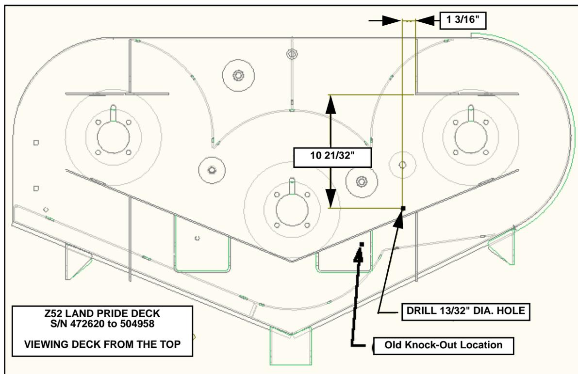
Z52 Baffle Mulch Kit Hole Relocation
