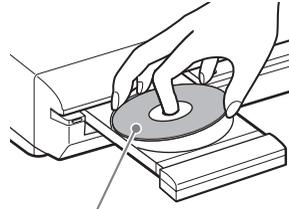
When you play an 8 cm disc, place it on the inner circle of the tray. Be careful that the disc is not skewed on the inner circle of the tray.
