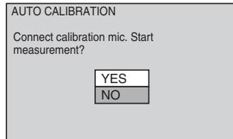
Connect the calibration mic to the A.CAL MIC jack on the front panel, and set it up at the ear level using a tripod, etc. (not supplied). The front of each speaker should face the calibration mic, and there should be no obstruction between the speakers and the calibration mic. Be quiet during the measurement.
