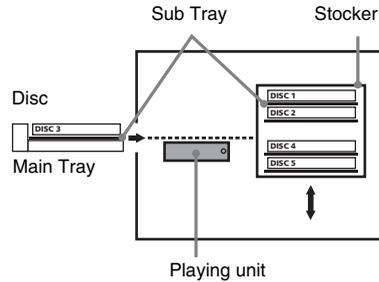
The disc changer consists of a playing unit and a stocker which transports the discs to the disc slot and the playing unit.
