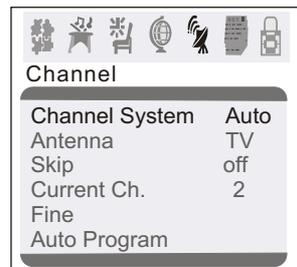
Channel System: Press the VOL(-/+ ) buttons to select the correct channel system. In general, you can set it as "AUTO" AUTO,NTSC and NTSC443 will display in turn
