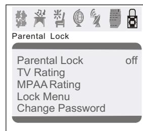
This function enables you to block certain TV channels in accordance to the V-CHIP requirement established by the FCC.
