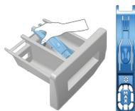
Clean the detergent drawer at regular intervals (every 4-5 washing cycles) as shown below in order to prevent accumulation of powder detergent in time.
