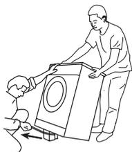
Tilt the machine backwards to remove the packaging reinforcement. Remove the packaging reinforcement by pulling the ribbon. Do not make this operation alone by yourself.
