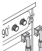
Connect the special water supply hoses supplied with the product to the water inlets on the product. Red hose (left) (max. 90 °C) is for hot water inlet, blue hose (right) (max. 25 °C) is for cold water inlet.
