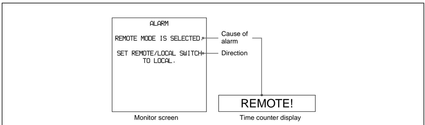
If such an alarm message appears, a connection or operation error may have been made, or condensation on heads may have occurred. Follow the direction indicated on the monitor screen.
