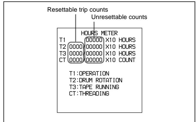
The four-digit value to the left of the slash (/) is the resettable trip count, and the right value is the cumulative total from manufacture.
