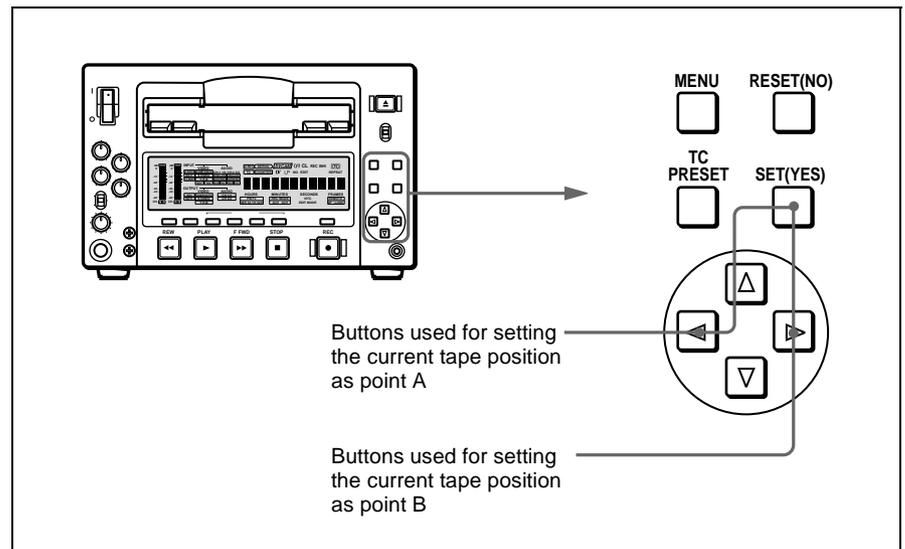
While holding down the SET (YES) button in the menu control section, press the ◀ or ▶ button. The time code value of the current tape position is set as point A or B, and a message "A set" or "B set" is displayed for 0.5 second in the time counter display.
