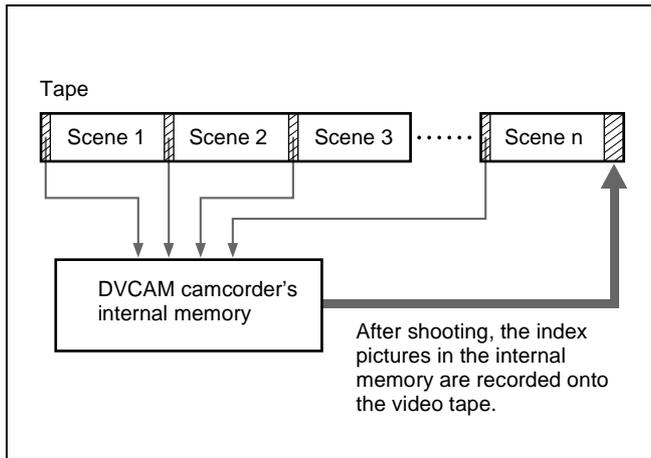
Up to 32 index pictures can be recorded onto the tape space normally occupied by one frame, as shown below.
