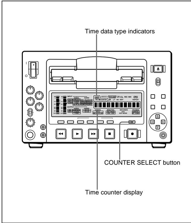
Press the COUNTER SELECT button on the front panel. Each press of this button cycles through three options: CNT value, time code, and user bit data. The time data type indicator for each option lights as it is selected.
