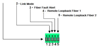
Note: Switch changes made when the product is powered up take effect immediately and will result in a link reset on both ports.
