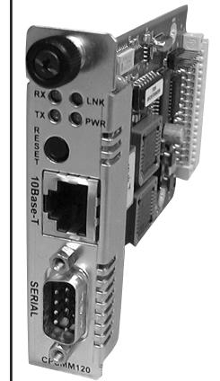
The CPSMM-120 includes Transition Networks **CPSMM100 firmware** embedded in the module, which can be accessed via the DB-9 serial port or the 10Base-T RJ-45 Ethernet port.
