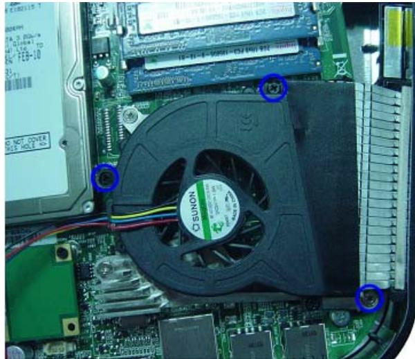
3. Lift CPU fan from CPU cooler.
