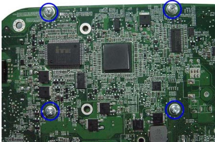
2. Remove HDD from Main board.
