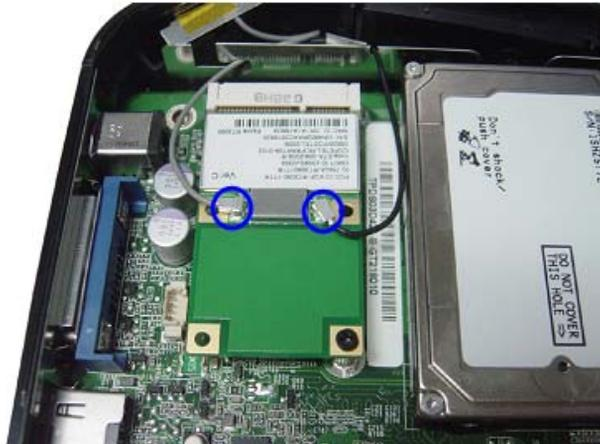
2. Use screwdriver to loosen the screw.
