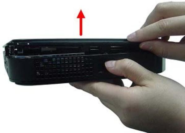
**WARNING:**Please be careful when open the cover,in order not to damage the EMI shielding.
