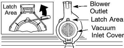
3. Gently tilt the handle of the screwdriver toward the back of the unit while pulling up on the vacuum inlet cover with your other hand.
