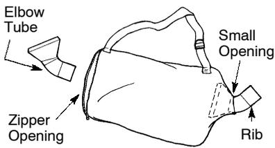
**NOTE:** Make sure edge of the small opening is flush against the flared area of the elbow tube, and the rib on the elbow tube is on the bottom.
