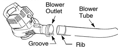
2. Tighten the tube clamp by turning the knob clockwise.
