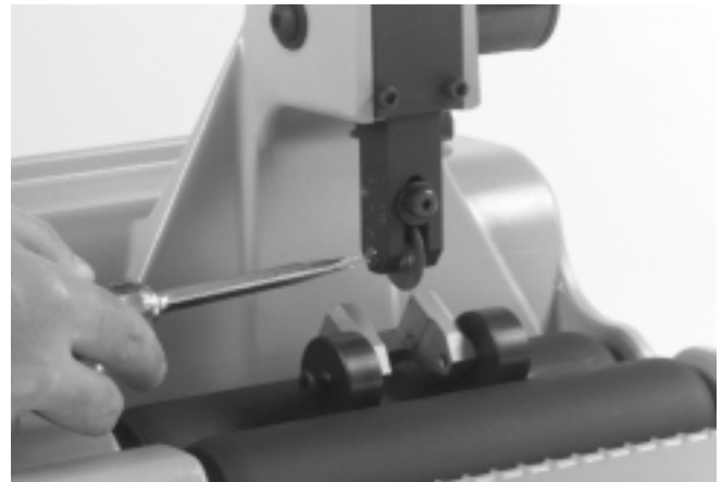
Figure 10B – Remove Cutter Wheel Screw
