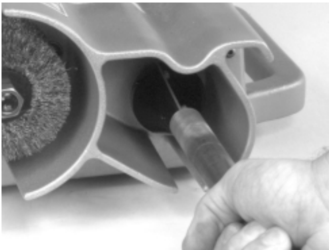
Figure 8 – Reaming I.D. of Tube
