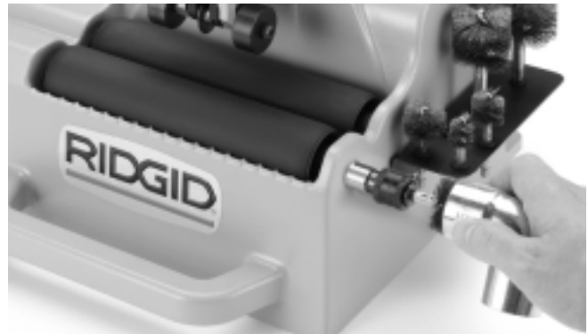
Figure 9 – Cleaning Inside of Fittings
