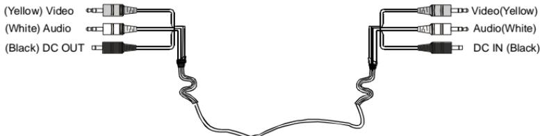
**NOTE:** The AVP Cable has different size plugs and colors at either ends. Pay carefully attention to ensure correct orientation. Do not force.
