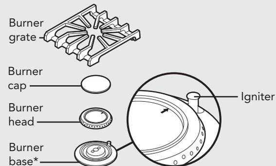
\* **Note:** When replacing burner head, arrow must be pointing towards back of range.
