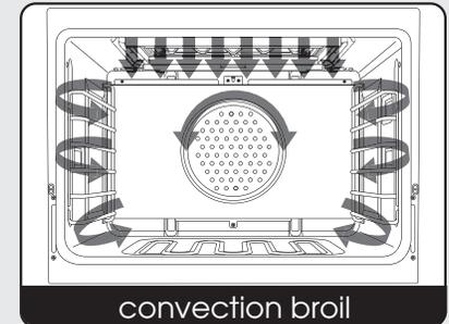
**\*Note:** This function uses a high-speed convection fan for optimum cooking performance. Some noise may be noticed from this high fan speed. This is normal.
