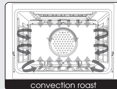
**\*Note:** This function uses a high-speed convection fan for optimum cooking performance. Some noise may be noticed from this high fan speed. This is normal.
