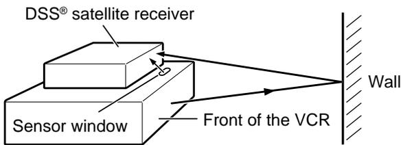
The infrared signals come out of the sensor window and the front of the VCR. Then they bounce off walls and other objects in the room and are received by the DSS® satellite receiver. The VCR sends out infrared signals to your DSS® satellite receiver even during timer program recording.
