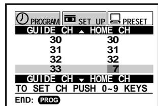
In some areas, one channel may be assigned more than one guide channel number. In this case, enter the home channel number to each of the guide channel numbers.
