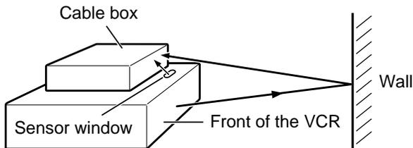
The infrared signals come out of the sensor window and the front of the VCR. Then they bounce off walls and other objects in the room and are received by the cable box.
