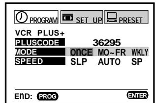
**4** Select “SPEED” using **CURSOR UP** or **CURSOR DOWN**, and set the recording tape speed.
