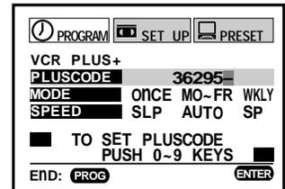
**3** Select “MODE” using **CURSOR UP** or **CURSOR DOWN**, and set the recording frequency.
