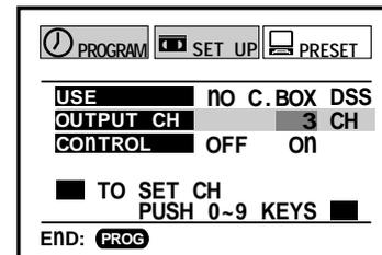
**6** Select "CONTROL" using **CURSOR UP** or **CURSOR DOWN**, and set to "ON" or "OFF" using **CURSOR RIGHT** or **CURSOR LEFT**.
