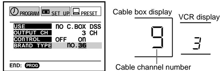
Make sure that the channel display of your cable box has changed to 9. If not, try each brand code assigned to the brand of your cable box until the display changes to 9.
