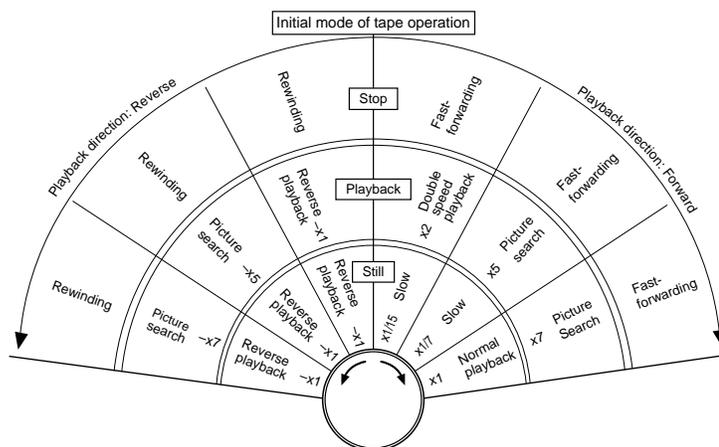
The playback speeds differ depending on the recording tape speed of the tape as follows.
