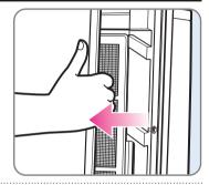
Separate filter that you want to Step2 replace from the filter case.
