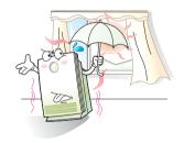
It should be installed more than 20<sub>cm</sub> away from walls or objects, and more than 30 ~ 60<sub>cm</sub> low from the ceiling. If it is too close to walls or objects, it could cause contamination in the surroundings.
