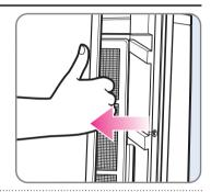
Please take out the plasma antibacterial catalysis filter, and then divide the filter into two pieces by pushing both hooks of the filter.
