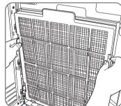
Please put the filters in the unit with Step3 the opposite direction, and then close the cover after filter replacement.
