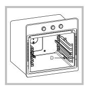
3. Secure the two frames with the guide rails using the holes provided on the oven walls (*see diagram*). The holes for the left frame are situated at the top, while the holes for the right frame are at the bottom.
