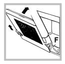
3. Grip the door on the two external sides and close it approximately half way. Unlock the door by pressing on the clamps **F**, then pull the door towards you, lifting it out of its slot (*see diagram*). To replace the door, reverse this sequence.
