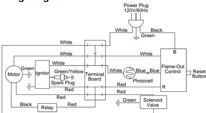
Figure 26 - Wiring Diagram
