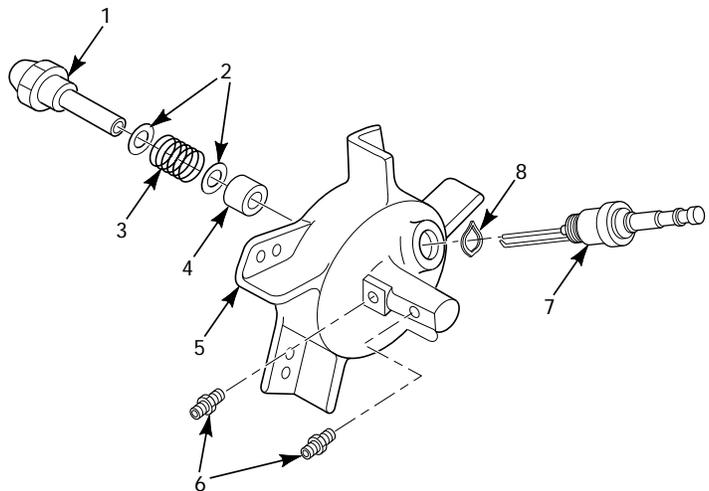
Figure 22 - Burner Head Assembly
