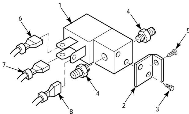
Figure 23 - Fuel Valve Assembly
