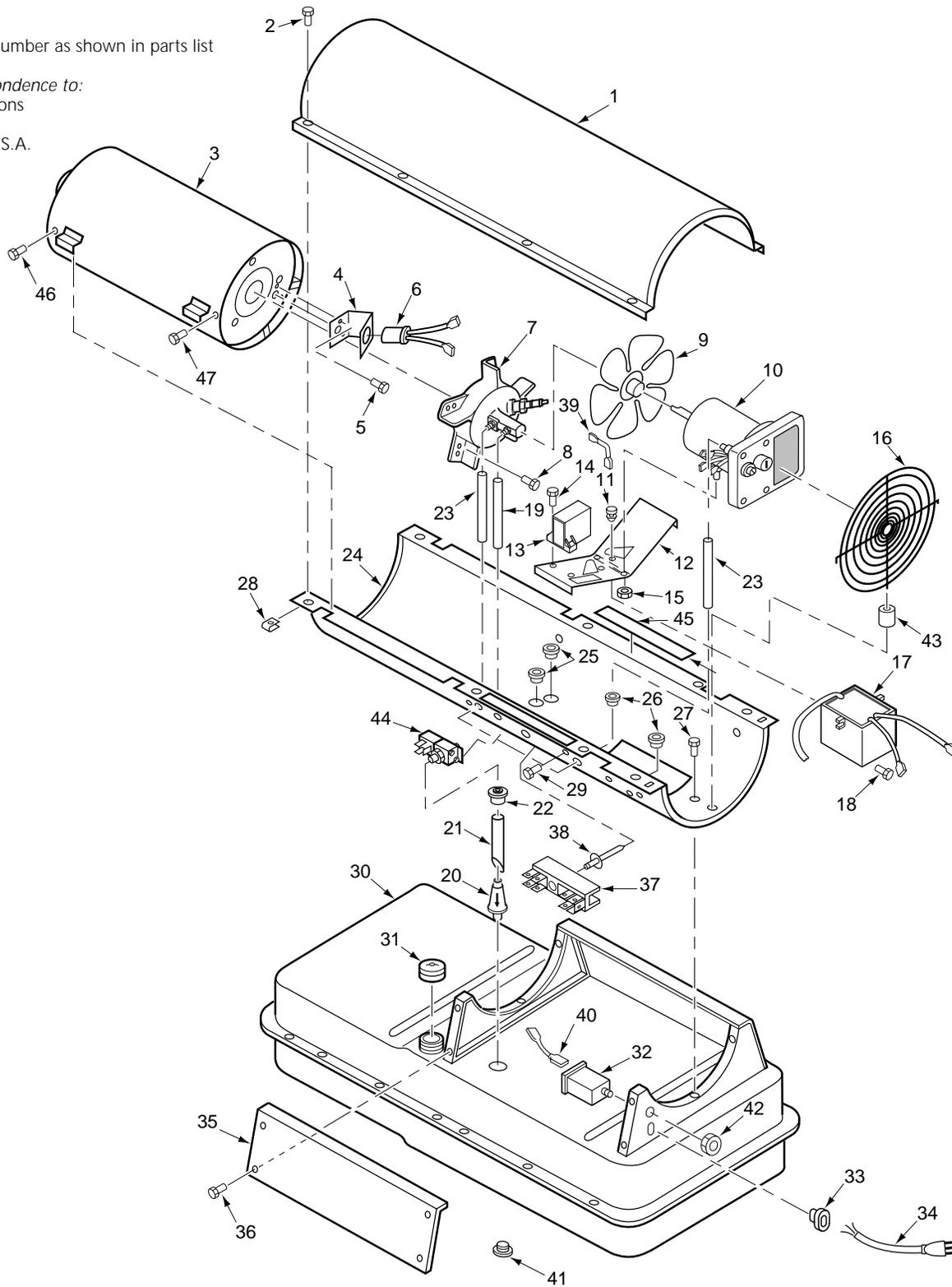
Figure 24 - Replacement Parts Illustration for Model 3VG79
