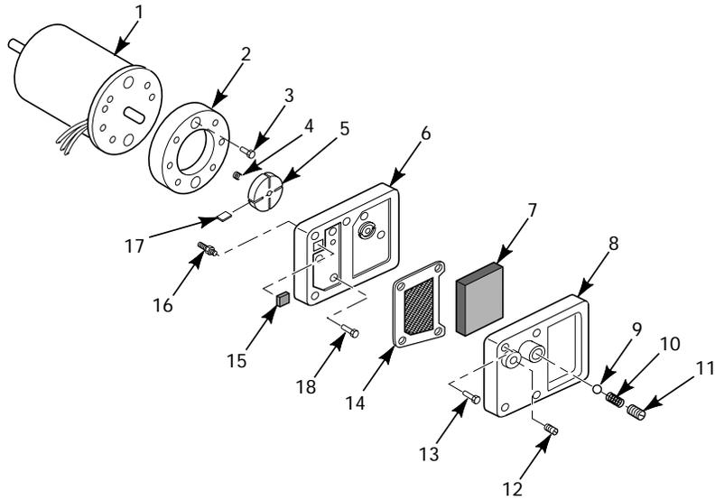
Figure 21 - Motor and Pump Assembly
