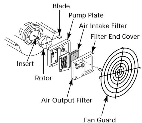
Figure 18 - Rotor Location
