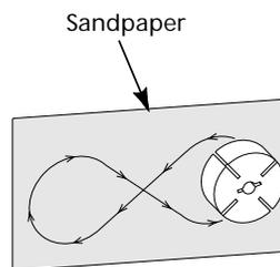
Figure 20 - Sanding Rotor
